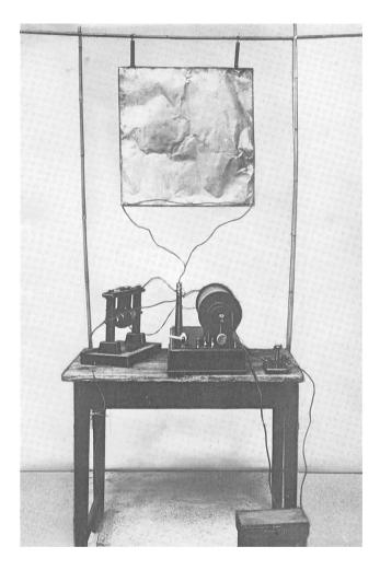
The first device developed by Marconi in Bologna in 1895 for wireless transmission. The antenna is a tin plate from an oil barrel. Another metal plate was laid on or buried in the ground. At the transmitting station, a spark gap (instrument on the table on the left) was connected between the two plates while at the receiving station the detector (a coherer, instrument on the table at the right) was connected between the plates.
